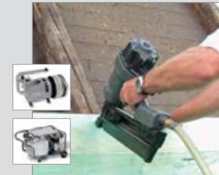
Straightforward, precise lath nailing
