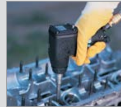
Impact wrenching for repair work
